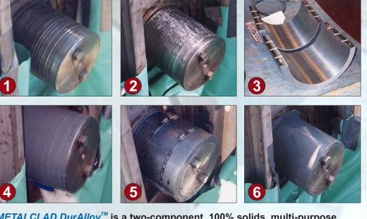
*METALCLAD DurAlloy*<sup>™</sup> is a two-component, 100% solids, multi-purpose polymer composite which can be easily machined on a lathe, drilled, tapped, filed, sanded and polished...
