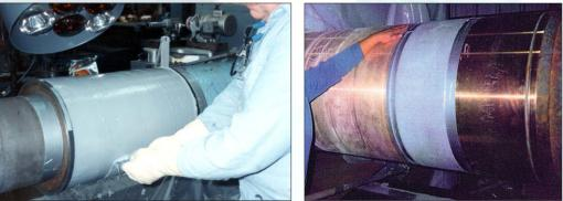
When properly mixed, *METALCLAD DurAlloy*<sup>™</sup> is a non-sagging paste which quickly cures to a metal-hard material creating a permanent bond to any rigid surface such as metal, plastic, glass, wood, concrete and more.
