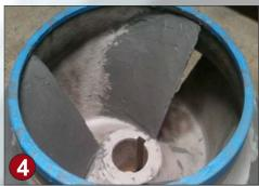
CeramAlloy® CP+AC is a paste when mixed, so it is easily applied. When cured, however, CeramAlloy® CP+AC becomes a metal-hard, ceramic-like compound. CeramAlloy® CP+AC is the best material to use when making repairs to areas deeply damaged by erosion/corrosion environments on all types of fluid flow equipment.
